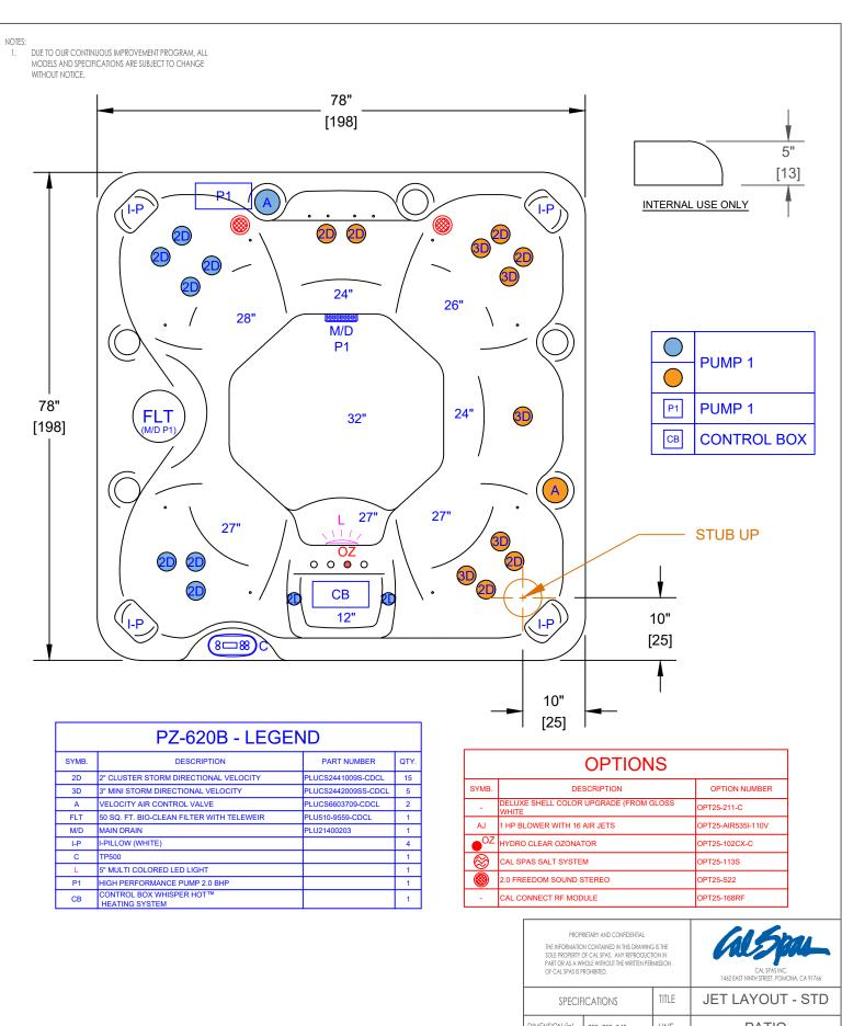
DIMENSION (in) 78"x78"x34" LINE **PATIO** 2025 SPA LINE DIMENSION (cm) 198x198x87 MODEL PZ-620B DRY WEIGHT 740 LBS [336 Kg] NUM Α FILLED WEIGHT 3577 LBS [1622 Kg] ČS003489 WATER CAP. 340 GAL [1287 L] SHEET 1 OF 1 SCALE
